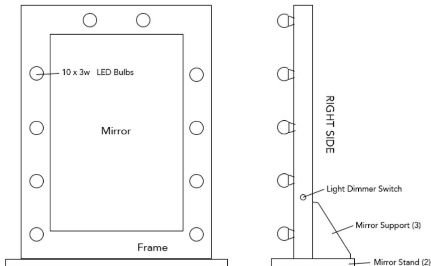
Fasten item 2 and 3 together using the four 44mm screws and washers provided. This creates the stand for the mirror.
